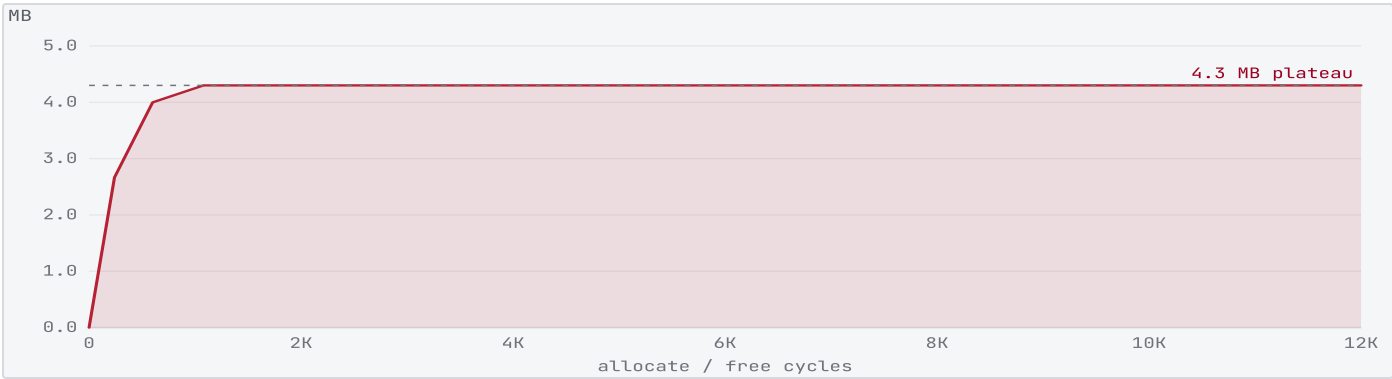
Fig. 5 Resident footprint across 12,000 cycles. Memory plateaus immediately and holds flat at 4.3 MB — recycled slots are reused in place, so steady-state churn commits nothing new.
