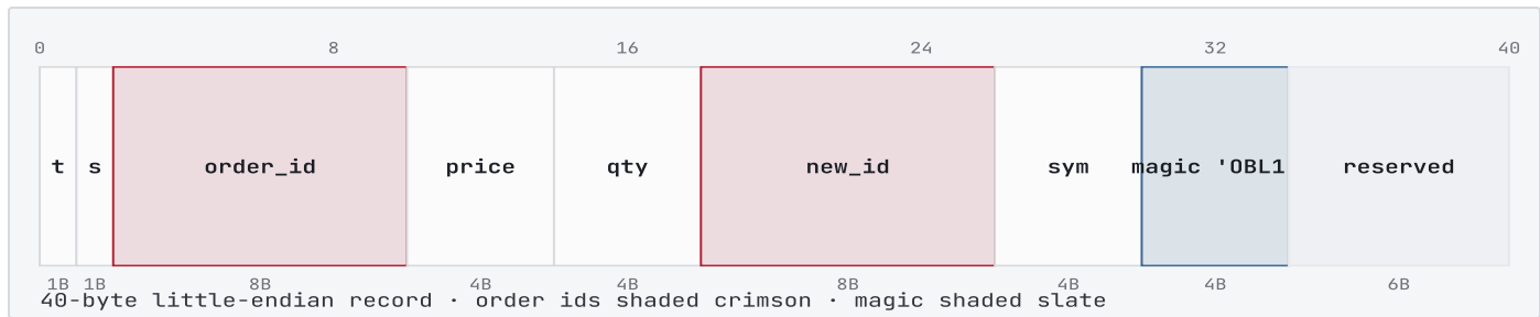
Fig. 1 The wire record. Order-id fields are shaded crimson, the 'OBL1' magic trailer slate. Decode validates the magic word and the type/side ranges before a message is admitted, so a corrupt frame is rejected rather than matched.
